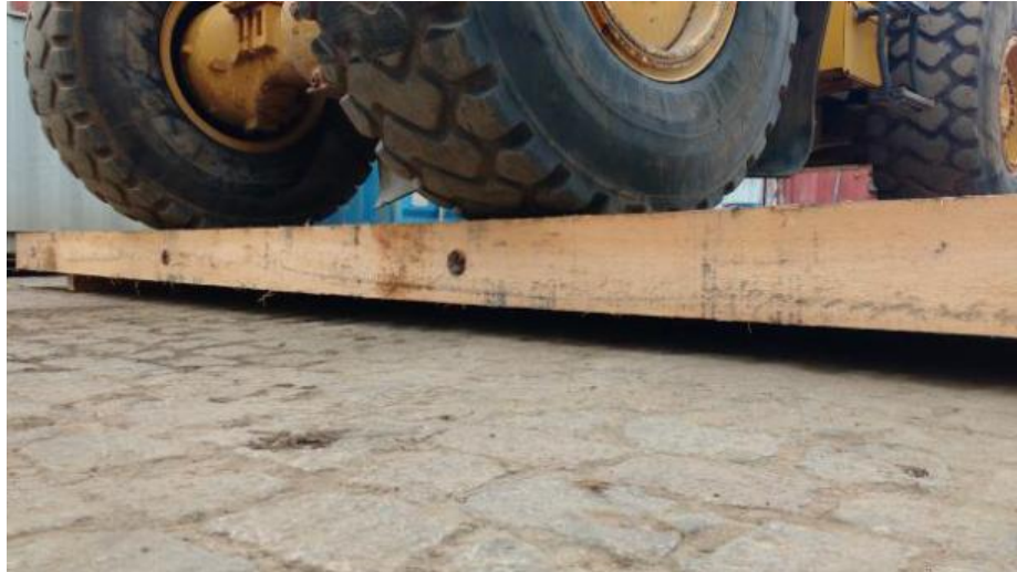
Figure 5 - Bending test of 18' x 8" x 48" Eucalyptus mat with 2x3 braces. No bending.
