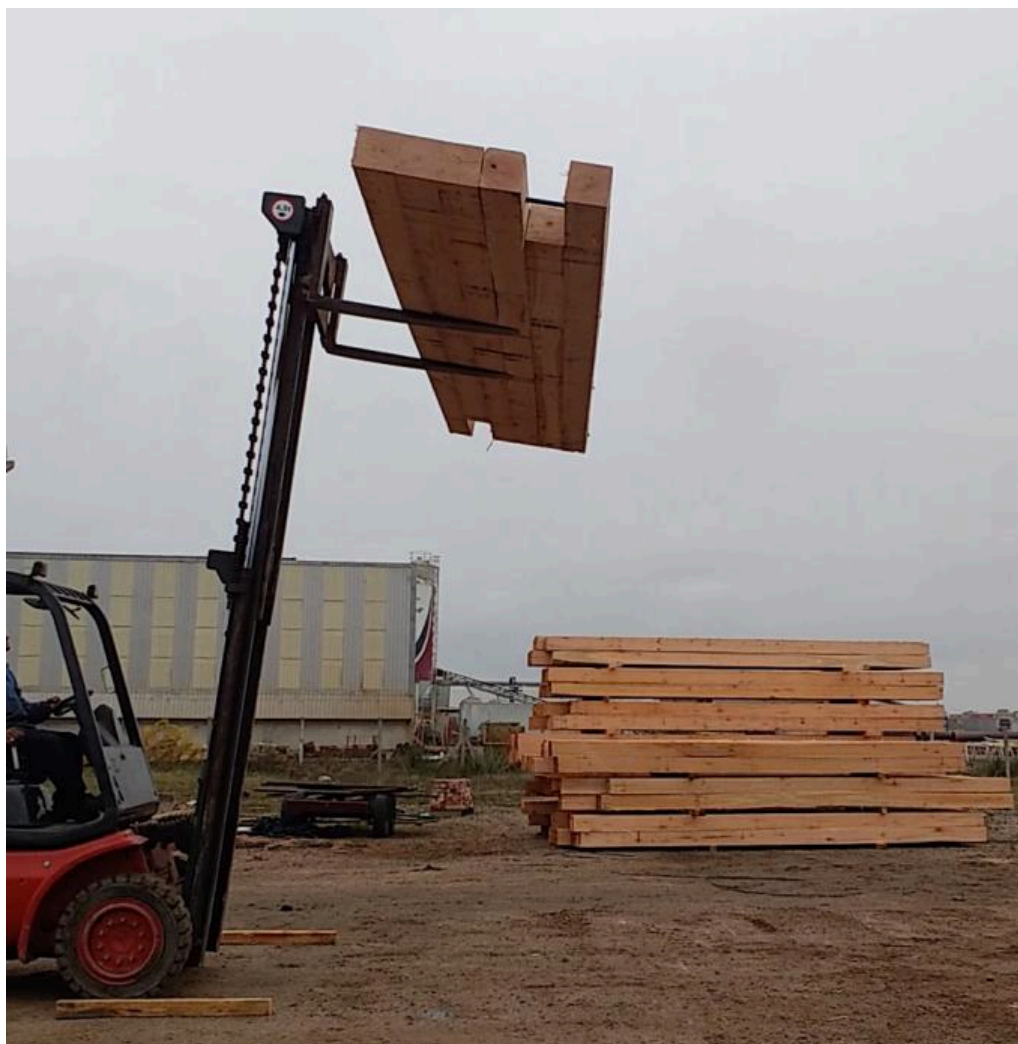
Figure 7 - Drop test from 16 feet onto hard soil. Mat was dropped 13 times before moving to Grade C mat.
