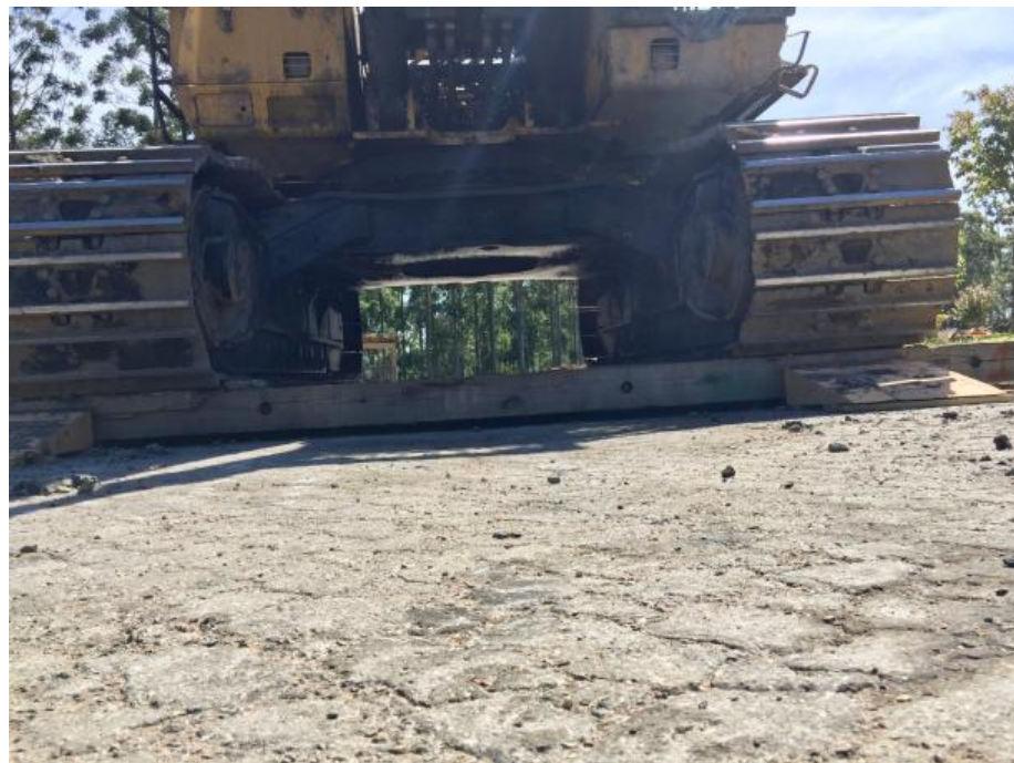
Figure 6 - Bending test with 150,000+ lbs. in bridging application of 18' x 8" x 48" mat. Mat flexed less than expected indicating Eucalyptus mats are as strong as engineer predicted.
