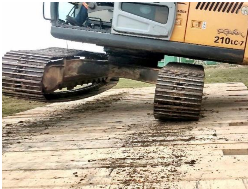
Figure 4 - Crawler on mats. Crawlers without grousers exert far less bending stress than wheel loaders.
